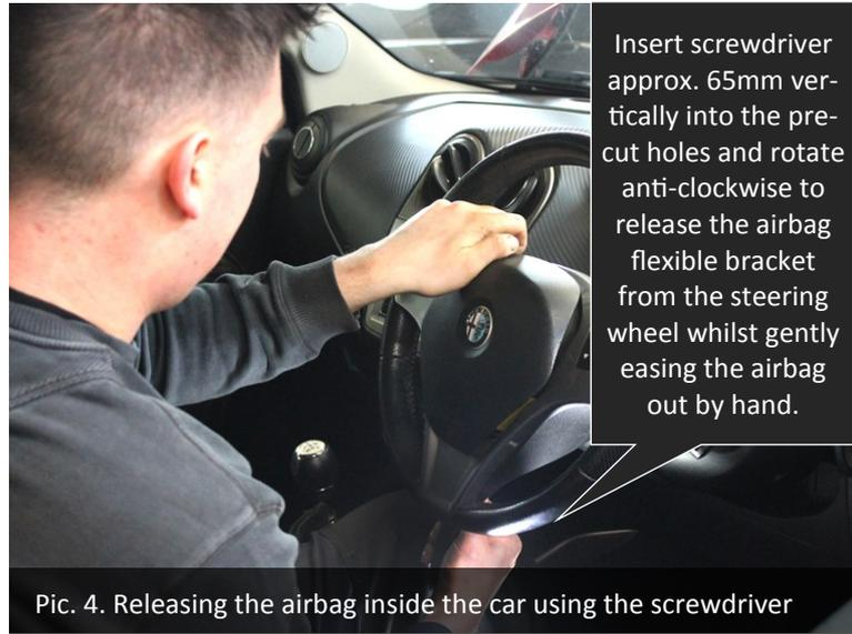
Pic. 4. Releasing the airbag inside the car using the screwdriver
